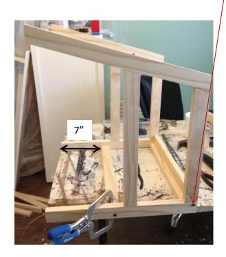
2d. Attach bottom front supports to legs, 7" up from bottom of the leg (keeping fronts flush) with glue and 2" finish nails. Follow up with a 2 1/2" self tapping screw, through the leg into the front apron from the outside, as shown in the picture
