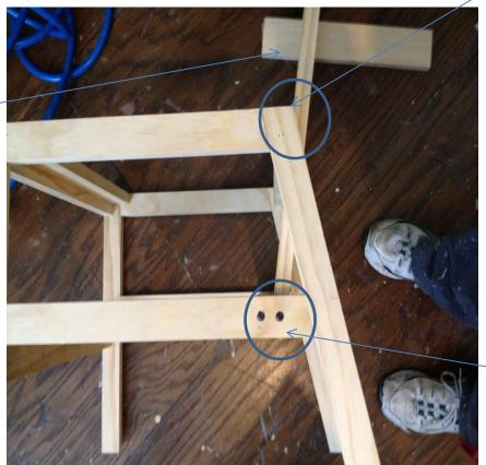
Bottom edge of chair back (back edge) lines up with bottom of lower support. Attach through support into bottom of back frame with 2 ½" screw. (this is why you didn't put a screw on this end when the back was assembled)
