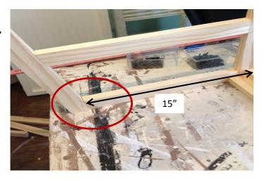
3c. Attach back apron to back legs, with front of the apron board lined up with the mark from above. Use 2" finish nails and glue. See picture.
